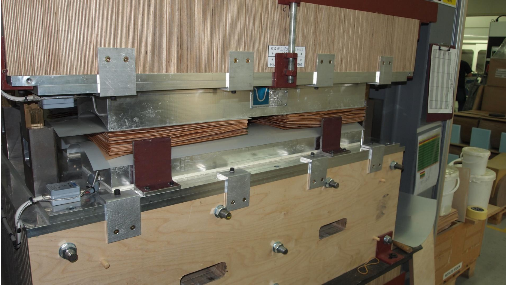
Birch under pressure in the gluepress
