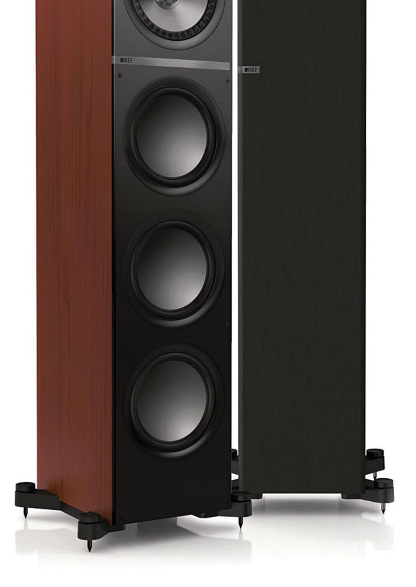
Uppermost on the front panel is the 8" Uni-Q driver, at its center a 1.5" vented aluminum-dome tweeter. This tweeter's size—the other KEF Q models have only a 1" dome—permits a lower crossover point from the mids to the highs: 1.8kHz vs 2.5kHz or higher. It is fitted with the Tangerine waveguide developed for KEF's Project Blade, to prevent untoward changes in dispersion at the crossover frequency and above. The
